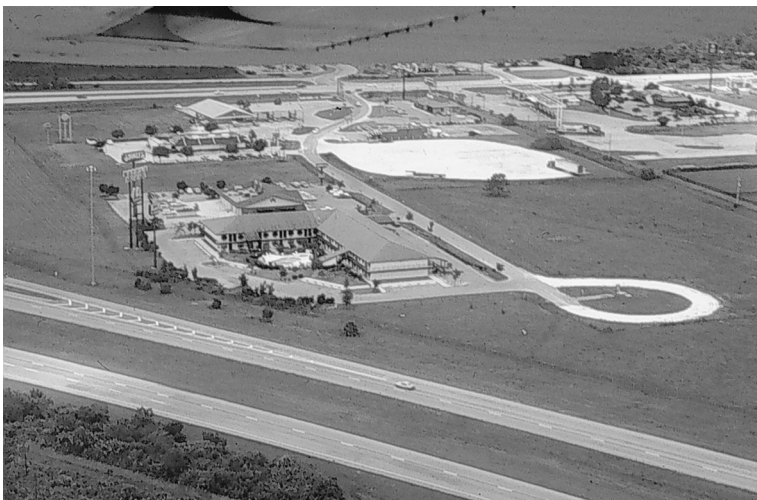
FIGURE 10-28 Service road perpendicular to the major roadway.
